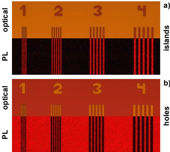
Figure 3. OLED patterns of 1 μm
