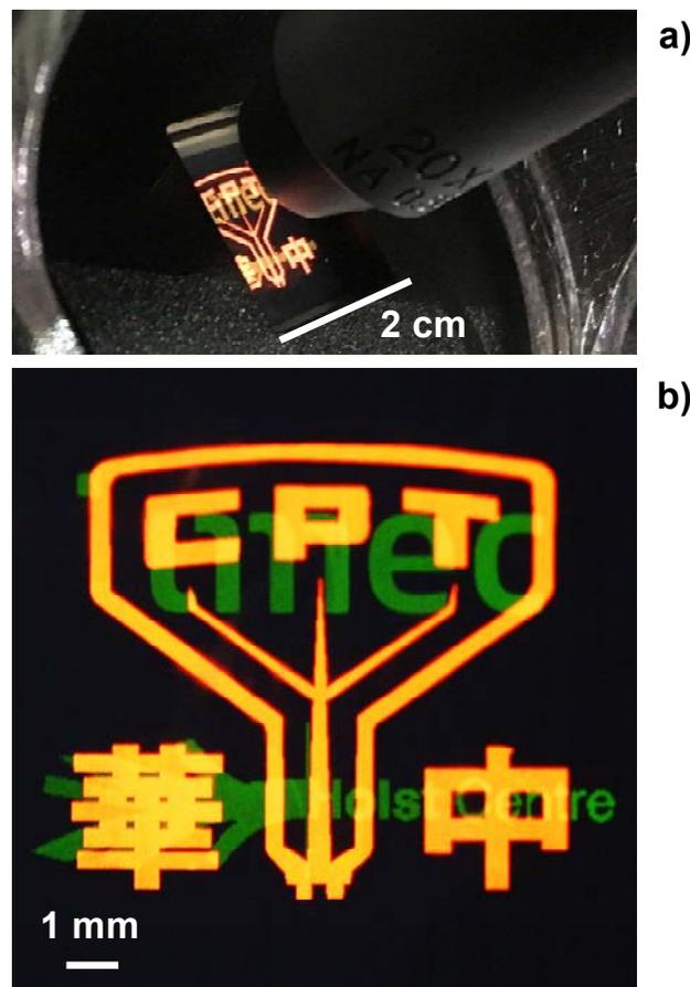
**Figure 8. Passive 1250 ppi patterned OLED display** 1400x1400 pixel array with 10 μm subpixel pitch and independent color driving: system view (a) and close-up of the active area during operation (b).
