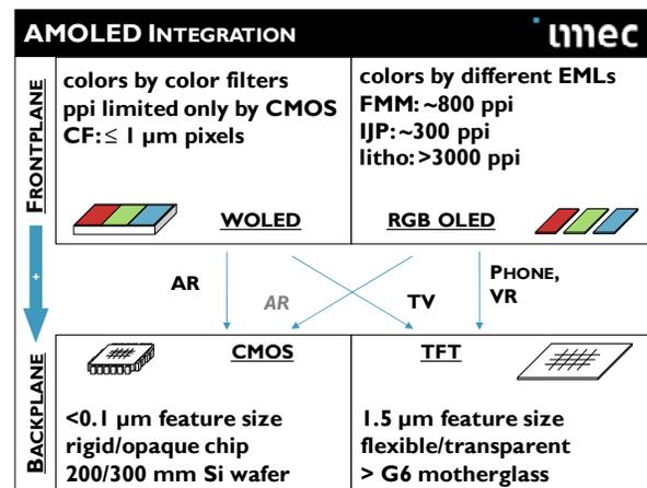
Figure 2. Integration options in AMOLED displays Color-by-white vs. RGB OLED frontplane can be fabricated on top of CMOS or TFT backplane. Each combination is suitable for different applications.
