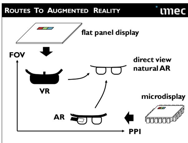
Figure 1. Head-mount display implementations Future augmented reality display should combine the benefits of both flat panel displays (size, transparency) and CMOS-based microdisplays (pixel density).
