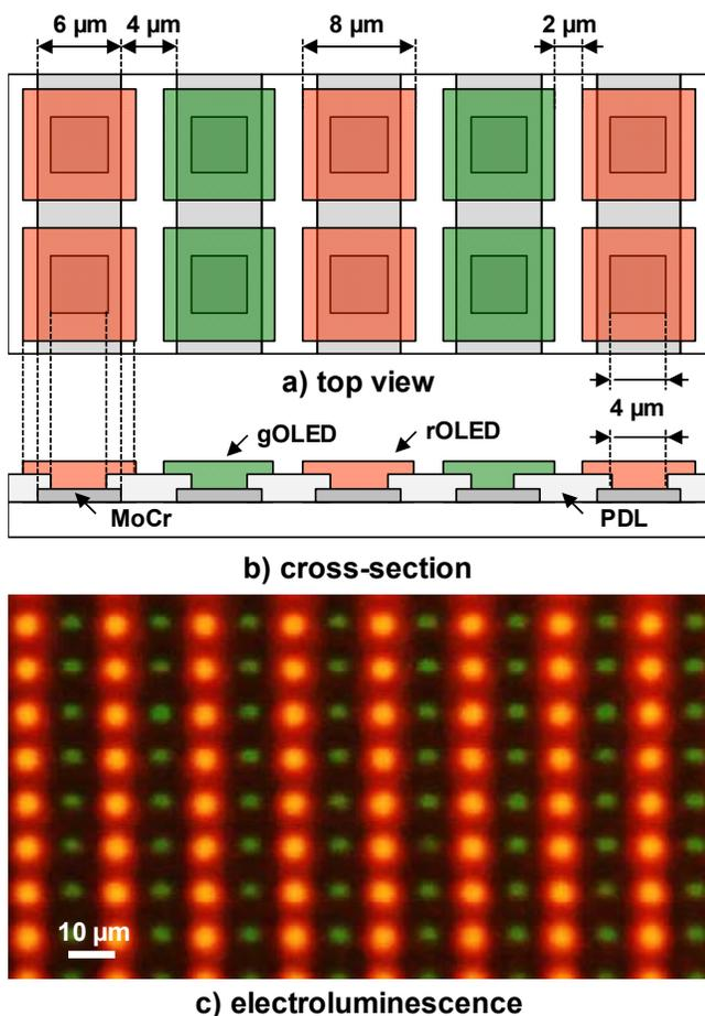
**Figure 7. Pixel design in a two color 1250 ppi display** Schematic top view (a) and side view (b) of a passive display designed for OLED patterning, with EL image of the working array (c).
